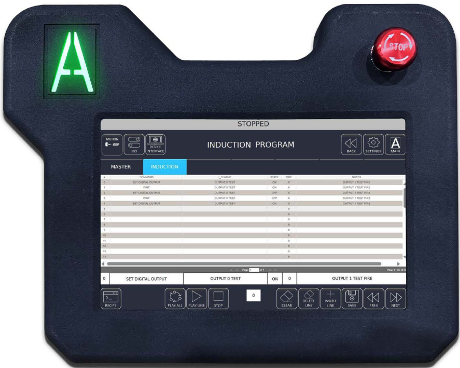
Picture: Teach Pendant Featuring the Induction Soldering Program
